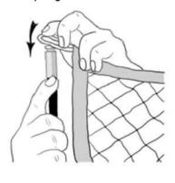
7. Take the last Black Rod and slot into Rod Coupling Tube.
